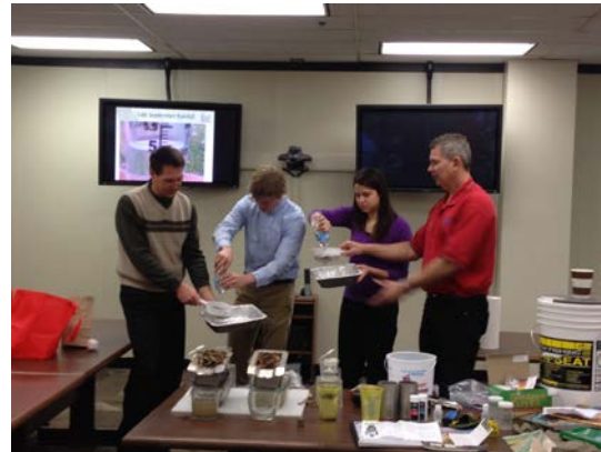
Mike Kucera (r), UNL Student Chapter members Bethany Brittenham and Tom Cowan and Doug Garrison (l) conduct an aggregate stability test on a no-till and conventionally tilled soil.
