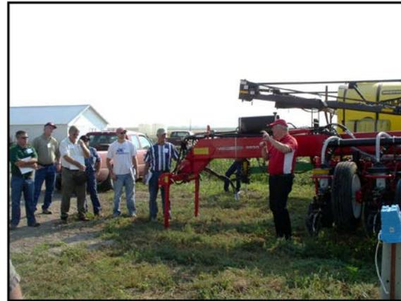
Paul Jasa, Extension Engineer, UNL explains the cutting power of a double disk opener for the No-Till systems. A No-Till system is more than just parking the equipment; we need to manage the residue. Four parts of a good system include
