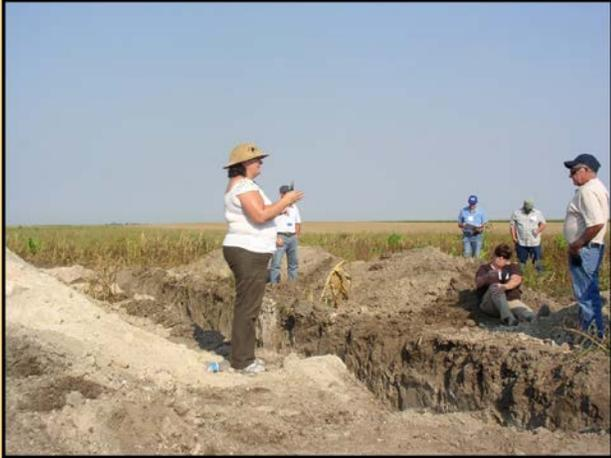
Odette Menard, Agricultural Engineer and Soil Conservationist from Saint-Hyacinth, Quebec Canada, explain the composition of the basic soil type. Soil is comprised of sand, silt and clay. The variations in the amount of each play a role in the qualities and characteristics of the soil.
