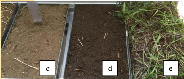
Before rain, (c) disturbed bare, (d) undisturbed (not tilled) bare, (e) undisturbed (grass) covered
