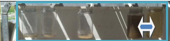
**Water runoff jars on pavement (water ran OFF soil pans)**
