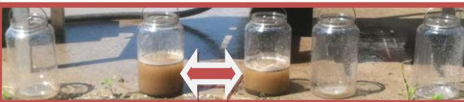
Infiltration is low on disturbed soils, high on undisturbed soils. Runoff low on covered and undisturbed soils, high on disturbed soils with less cover.
